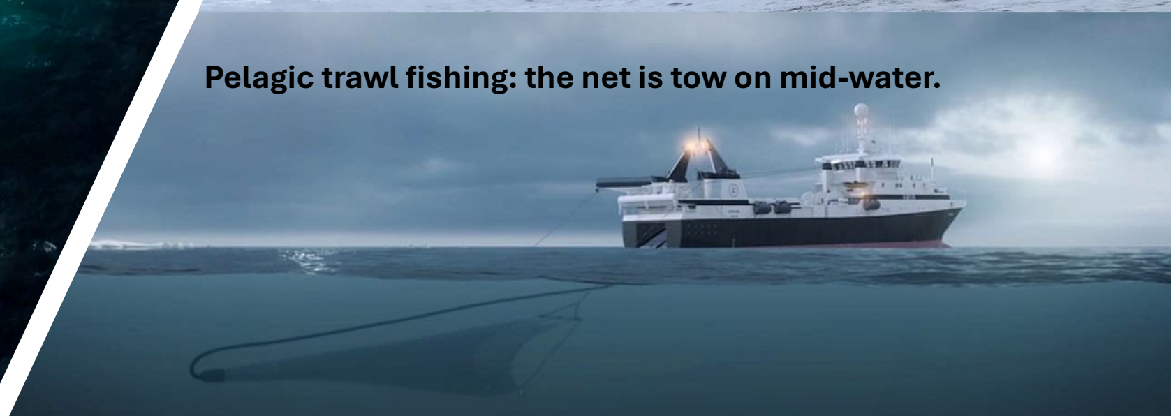
Stern-trawler tow the net from the back of the vessel.
